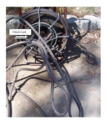
The damage to this snake cable was caused completely from misuse.
